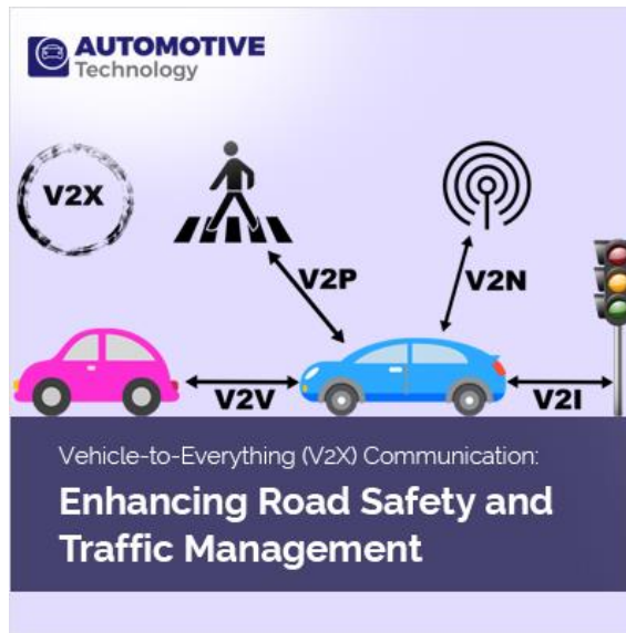
Figure 1: V2X communications that allow an AV to operate safely. (Source: Automotive Technology)
